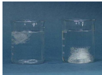
FIGURE 43 Frozen D_2O (At Right) Sinks in Light Water While Frozen H_2O Floats.
