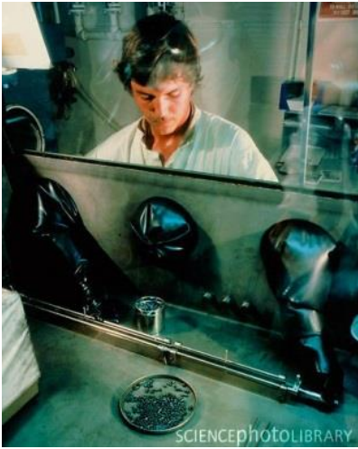
FIGURE 27 A Technician Arranges Fuel Pellets in a Trough Before Sliding the Cladding Over Them.
