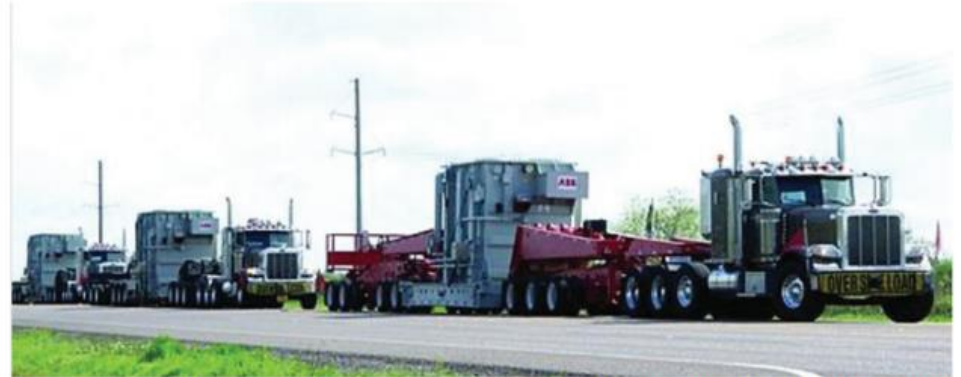
FIGURE 6.3 Three ABB single-phase 345 kV compact replacement transformers being moved from St. Louis, Missouri, to a substation in Houston, Texas, under a Department of Homeland Security demonstration project. SOURCE: DHS (2012).
