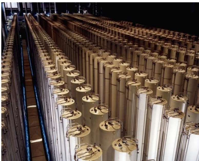
FIGURE 19 Gas Centrifuge Cascade
