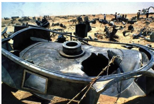
FIGURE 14 EMIS "Calutron" Discovered in Iraq in 1991
