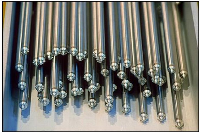
FIGURE 28 Completed Fuel Rods
