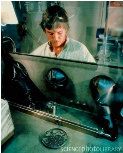
FIGURE 27 A Technician Arranges Fuel Pellets in a Trough Before Sliding the Cladding Over Them.
