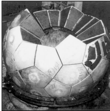
Figure 10: Explosive Lenses Arranged in Soccer Ball Shape
