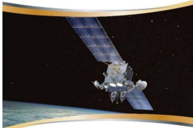
The Advanced Extremely High Frequency, or AEHF, system provides survivable, global, secure, protected and jam-resistant communications for high-priority military ground, sea and air assets. (U.S. Air Force photo)
